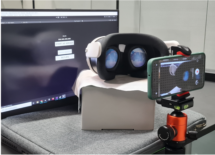
FIGURE 4.3: In-Situ MTP Measurement Setup at the IXLab
